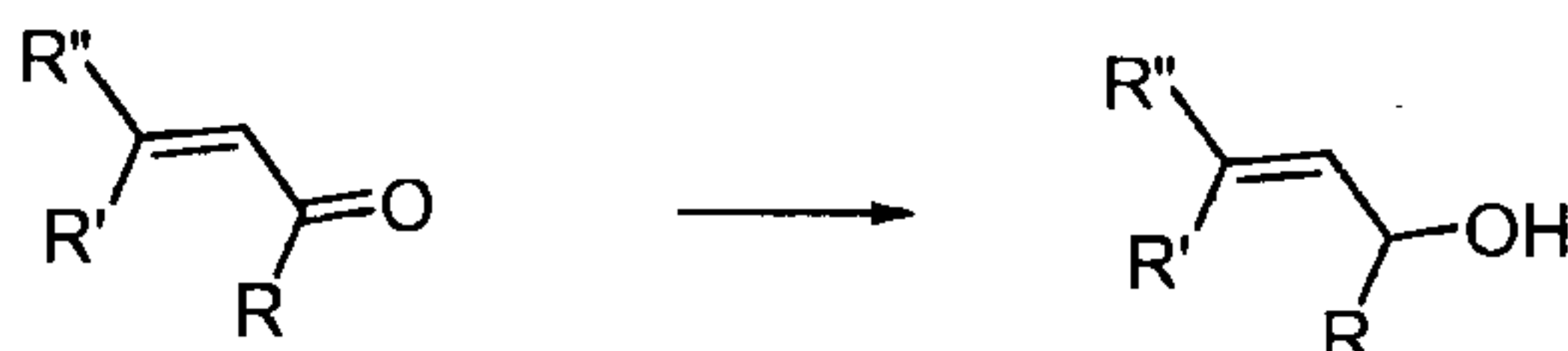
Scheme 39: Reduction of an \alpha,\beta -unsaturated ketone to an allylic alcohol (General Procedure MM)
