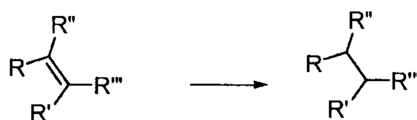
15 Scheme 30: Hydrogenation of an alkene (General Procedure DD)
