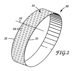
This invention relates to an abrasive article (e.g., sheet or belt) having a plurality of ridges of abrasive material deployed on a surface thereof so as not to be aligned with its machine direction and to methods for making the same.
