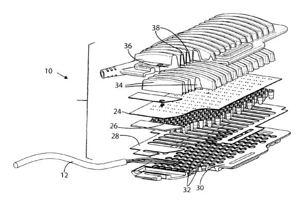
(57) Abstract: A light treatment head which incorporates an array of light sources, a flexible power distribution panel, a plurality of heat sink bodies closely associated with the light sources, and a flexible housing enclosing the light sources, the distribution panel and the heat sink bodies.
