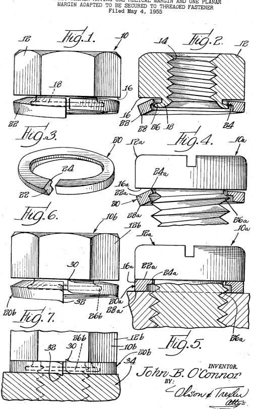
Jan. 29, 1957 J. B. O'CONNOR 2,779,375 SPLIT WASHER HAVING ONE HELICAL MARGIN AND ONE PLANAR MARGIN ADAPTED TO BE SECURED TO THREADED FASTENER Filed May 4, 1955
