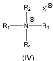
wherein  $R_1$ ,  $R_2$ , and  $R_3$  are independently  $C_1$  to  $C_{20}$  alkyl,  $R_4$  is methyl or benzyl, and  $X^-$  is a halide or methosulfate.
