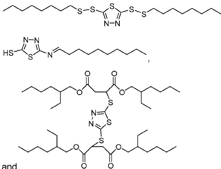
**[0046]** The compound of Formula I or II and the compound of Formula III or IV can be present in the anticorrosion composition at a concentration of from 5 to 95 wt.% and 95 to 5 wt.% respectively, based on the total weight of the formulation. Preferably, the compound of Formula I or II and the compound of Formula III or IV can be present in the anticorrosion composition at a concentration of from 5 to 30 wt.%, and 30 to 5 wt.% respectively, based on the total weight of the formulation.
