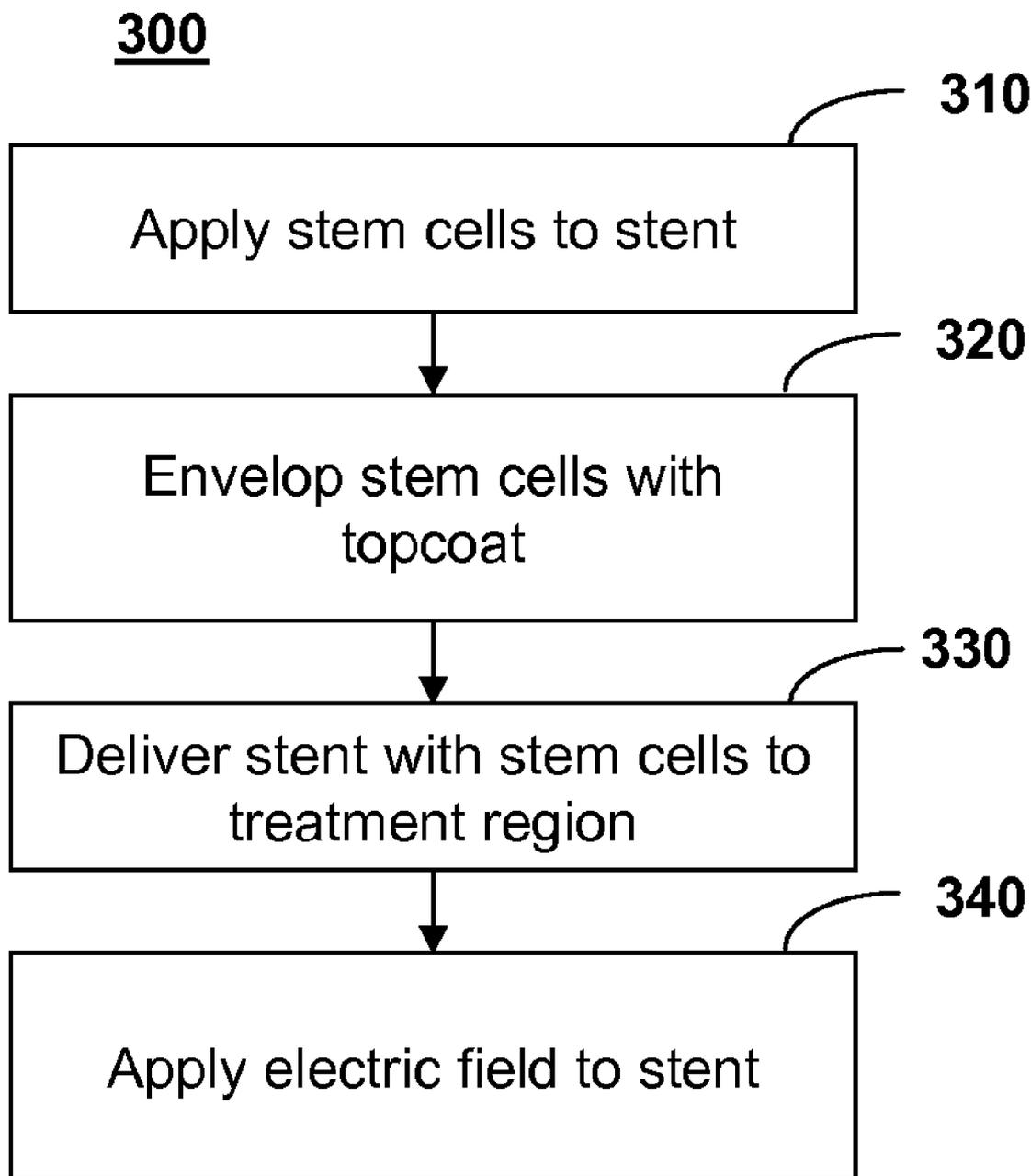
**STEM CELL COATED STENT**
