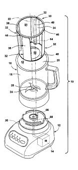
housing and a magnetic blade member in the wiper assembly. The operable coupling between the motor and the wiper assembly results in rotation of the wiper blade when the motor is activated, which removes food from the inner wall surface of the food blending chamber during rotation.
