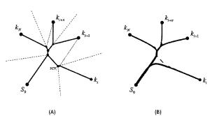
sink or one source; and where the intersections of Voronoi cells are Voronoi cell vertices; locating a sink endpoint centroid; connecting a source to a nearest Voronoi cell vertex; connecting at least one sink to at least one of the remaining Voronoi cell vortices to complete the network; and performing a smoothing function on the network to form a smoothed network.
