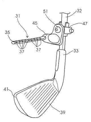
(57) Abstract: Apparatus (31) having housing (45) affixed to club clamp (47) for attachment to shaft (32) of club (33) is used for analzyzing a golf swing. Housing (45) is affixed to clamp (47) at pivot (51) so that row (35) of elements (37) can be rotated relative to a viewer and, in combination with clamp (47) adjusted to extend parallel to and a selected distance above golf club head (41) having club face (39).
