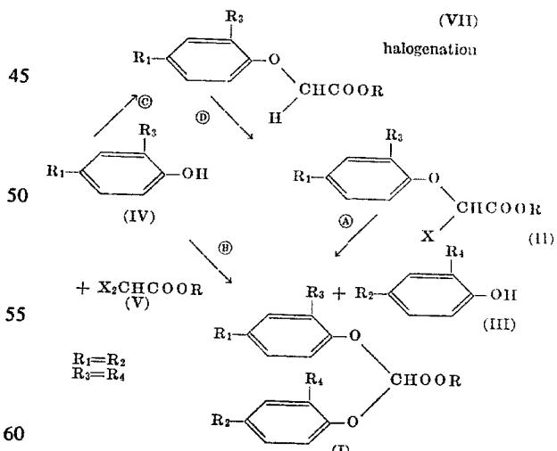
where  $R$ ,  $R_1$ ,  $R_2$ ,  $R_3$  and  $R_4$  are as defined above, and  $X$  represents halo, preferably chloro or bromo.
