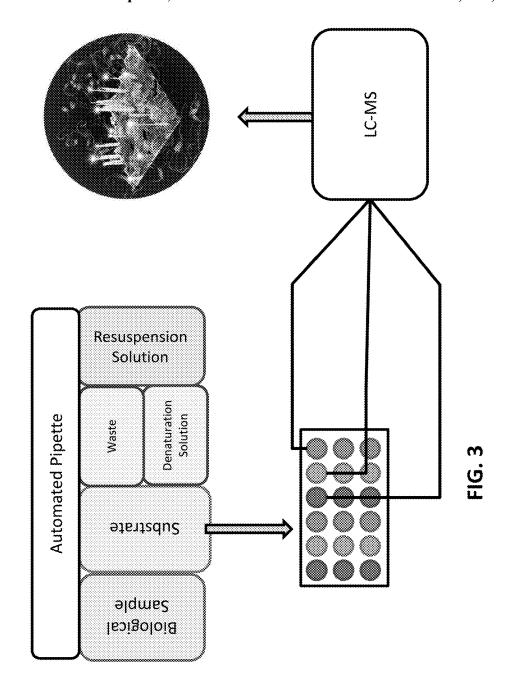
Transferring sample into substrate partition with sensor array
