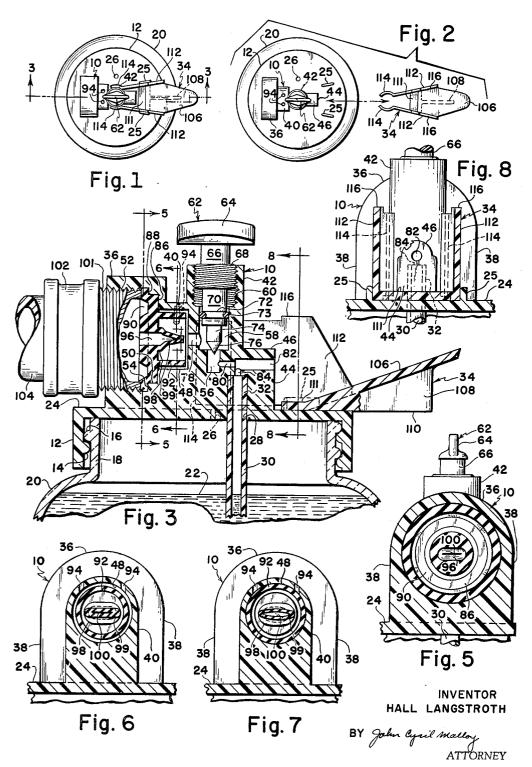
SPRAY HEAD HAVING A VALVE STEM AND DISC-FORM CHECK VALVE
