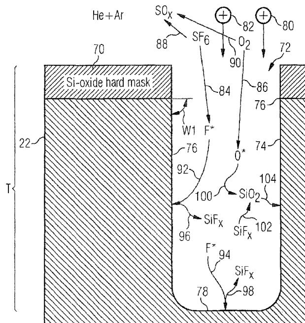
(57) Abstract: The invention relates to a method, wherein plasma is used for energetic excitation of a reactive etching gas. The reactive etching gas is a component of a continuous gas flow. A recess is deepened by at least 50 micrometers without interrupting the gas. A simple method is thus disclosed in order to produce deeper recesses.
