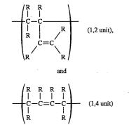
wherein each R is independently a hydrogen, lower alkyl ( $C_1-C_5$  hydrocarbon), halogen or substituted or unsubstituted aromatic radical. It is often preferred that R is hydrogen so that the polymer backbone is polybutadiene.
