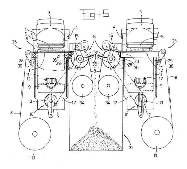
The invention relates to an apparatus for brewing a drink, such as coffee, comprising a chamber for accommodating a mixture of water and a ground product to be extracted, 5 which chamber has a perforated base on which a strip of filter material can be laid, means being provided on one side of said base for moving the strip of filter material over the base after a quantity of drink has been brewed and removed via the piece of filter material and the base located beneath 10 it
