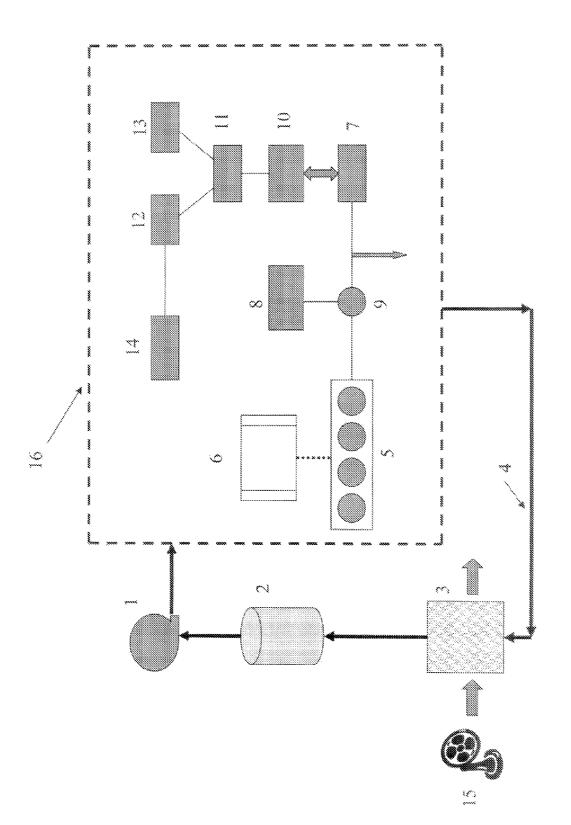
Figure 1. Schematic diagram of an illustrated example of a hybrid vehicle cooling system
