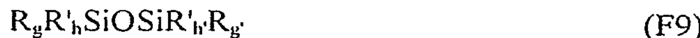
where  $R$ ,  $R'$ , are as defined above, the sum of  $h$  and  $h'$  is an integer with a value of 5 at least two; the sum of  $g$  and  $h$  is equal to 3; and the sum of  $g'$  and  $h'$  is equal to 3. For example, there are included as disiloxanes of formula (F9), 1,1-divinyl-tetramethyldisiloxane, 1,3-divinyltetramethyldisiloxane, hexavinyldisiloxane, 1,1,3-trivinyltriethyldisiloxane, 1,1,3,3-tetravinylmethyldisiloxane, 1,3-divinyl,-1,3-dimethyl,-1,3-diphenyldisiloxane, etc.
