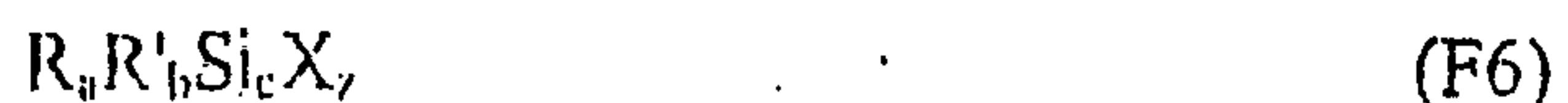
where R is free of aliphatic unsaturation and selected from monovalent hydrocarbon radicals, R' is selected from monovalent aliphatically unsaturated hydrocarbon radicals, X is a hydrolyzable radical, c is an integer having an average value of at least 1, b is an integer having an average value greater than or equal to 2, and the sum of a plus b plus z equals the sum of 2 and two times c for a linear or branched silane and the sum of a plus b plus z equals two times c for a cyclic silane;
