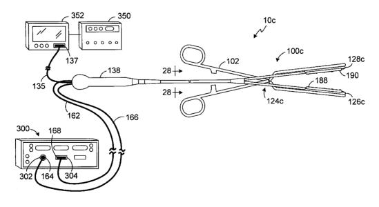
2006/086063 A3 ||||||||||||| (57) Abstract: An apparatus including a tissue coagulation device that creates a current path And a stimulation electrode carried within the current path. The stimulation electrodes may be used to perform a variety of functions before, during and after lesion formation procedure. For example, to confirm tissue contact, to evaluate the lesion and to confirm whether or not a therapeutical lesion has been formed.
