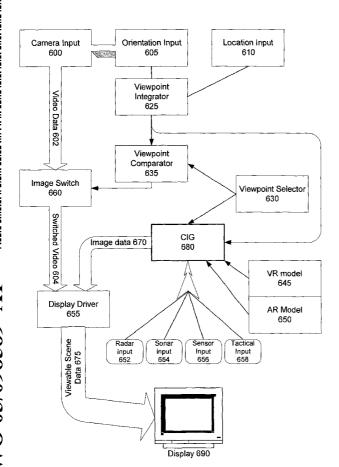
(57) Abstract: A combination of interacting virtual reality (VR) and augmented reality (AR) system is provided where the system automatically switches from VR to AR when the user selected viewpoint coincides, within tolerance, with the observable AR viewpoint. The invention discloses an apparatus adapted to provide easy acces and automatic switching between AR and VR, and method therefor.
