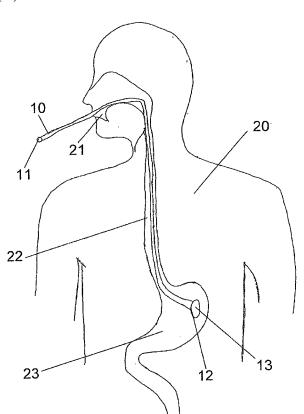
(57) **Abstract**: The invention relates to a gastric tube assembly comprising a tube with first and second ends and a lump element attached to the second end of the tube, wherein the tube and the lump element are dissolvable, said lump element being configured to be swallowed by a patient, thereby feeding said tube through the patient's oesophagus.
