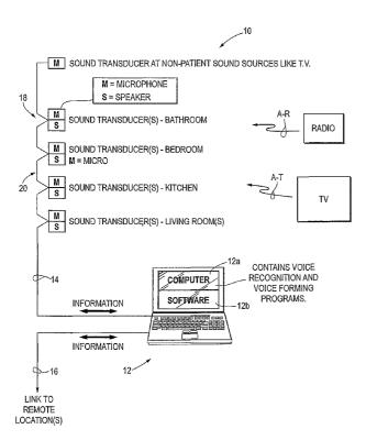
(57) Abstract: A system for monitoring conditions associated with an individual in a region includes at least one speech input transducer and speech processing software coupled thereto. Results of the speech processing can initiate communications with a displaced communications device such as a telephone or a computer to provide a source of feedback.
