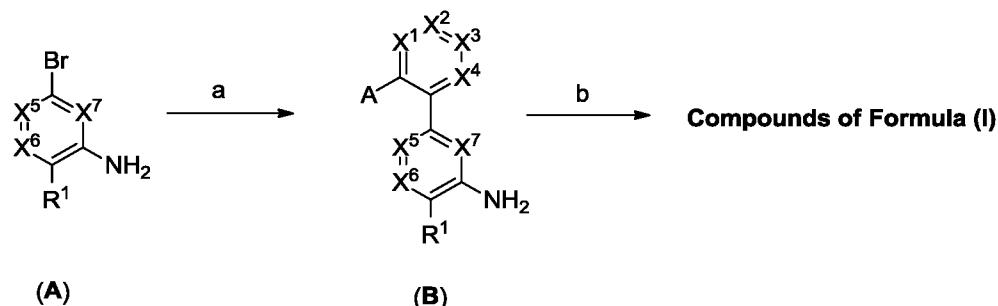
**Scheme 1:** a)  $R^aB(OH)_2$  or boronate ester,  $Pd(Amphos)Cl_2$ ,  $K_3PO_4$ , dioxane/ $H_2O$ ,  $\mu$ wave,  $110^\circ C$ ; b)  $R^2C(O)OH$ , coupling agent or  $R^2C(O)X$ , where  $X$  is a halide, amine;
