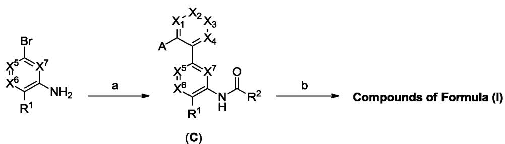
**Scheme 2:** a)  $\text{R}^2\text{C(O)OH}$ , coupling agent or  $\text{R}^2\text{C(O)X}$ , wherein X is a halide amine;
