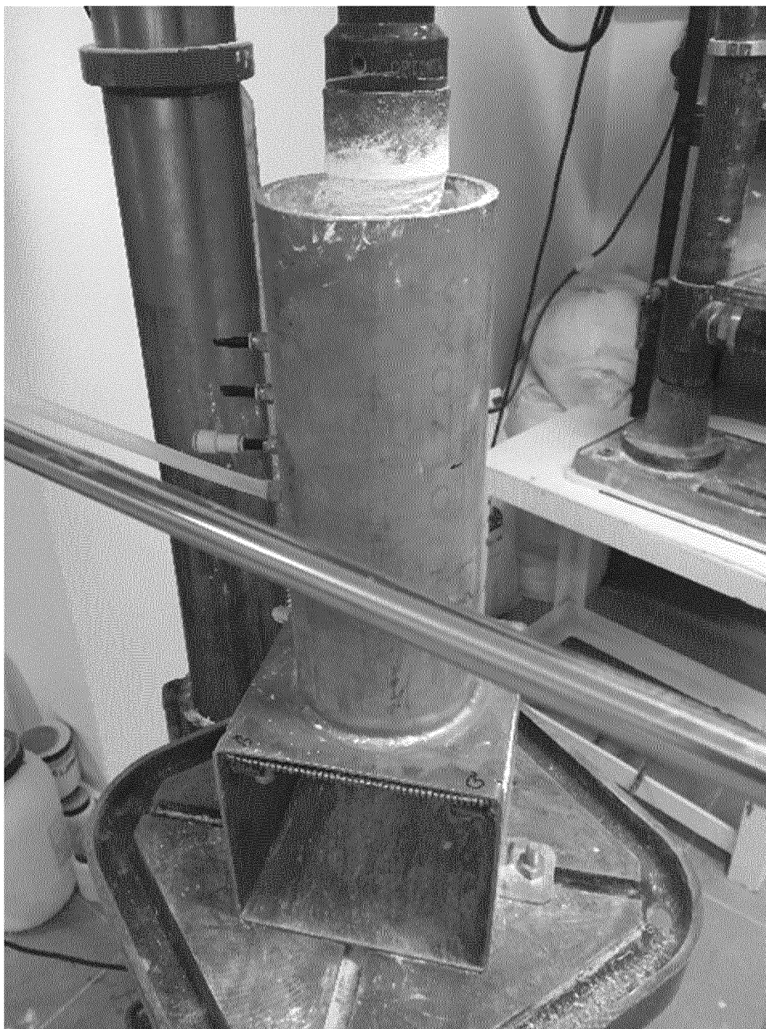
Figure 4: Photograph of a system for producing nano-PCC comprising one dry sandmill and inlets A), B) C) and outlet D)
