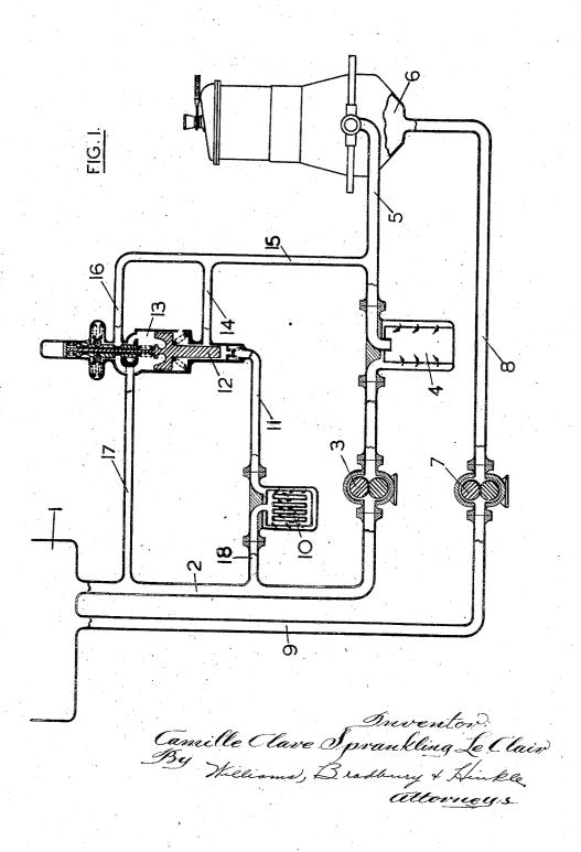
LUBRICANT CIRCULATING SYSTEM INCORPORATING FILTERING MEANS
