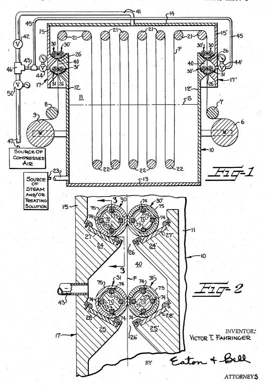
APPARATUS FOR SEALING A PRESSURE VESSEL
