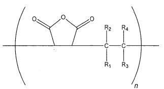
wherein n is one or greater;  $R_1$ ,  $R_2$ ,  $R_3$  and  $R_4$  are selected from hydrogen, methyl and polyisobutyl having at least about 30 carbon atoms (preferably at least about 50 carbon atoms) wherein either  $R_1$  and  $R_2$  are hydrogen and one of  $R_3$  and  $R_4$  is methyl and the other is polyisobutyl, or  $R_3$  and  $R_4$  are hydrogen and one of  $R_1$  and  $R_2$  is methyl and the other is polyisobutyl. The polyPIBSA copolymer may be alternating, block, or random.
