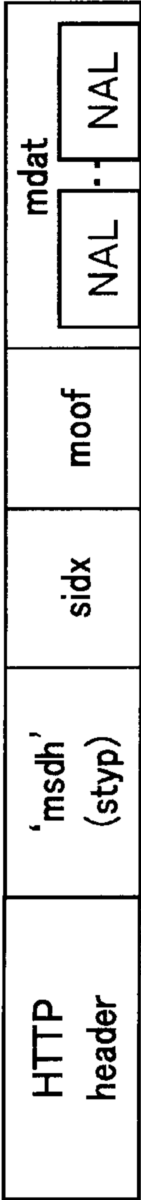
(a) SUB GOP MEDIA SEGMENT STORAGE HTTP PACKET CONFIGURATION EXAMPLE 1
