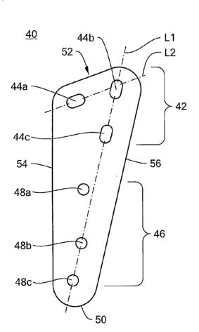
(57) Abstract: A fixation plate with a base section including apertures for fixation to one bone segment and a leg section extending from the base section and including apertures for fixation to another bone segment. The expanse of the base section tapers gradually to smoothly cojoin with the leg section and the expanse of the leg section continues to taper to a distal rounded end of the leg section.
