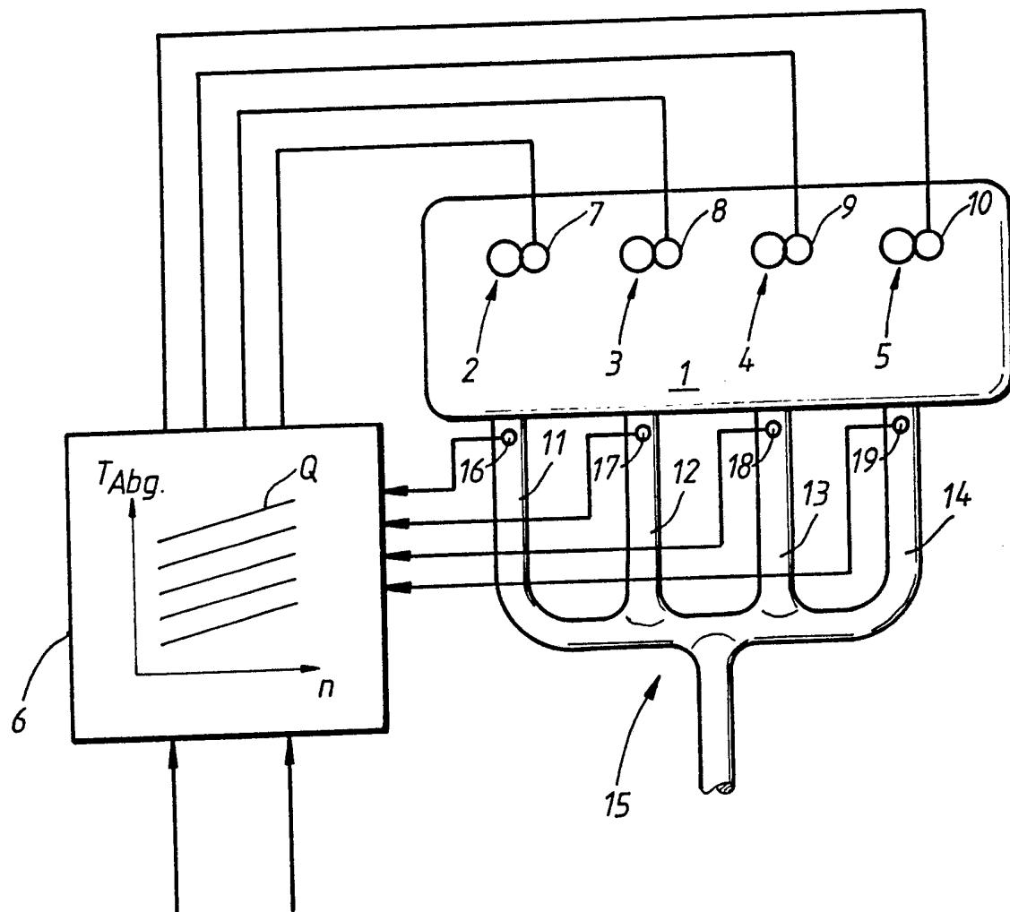
Process for Regulating the Injection Quantity on a
