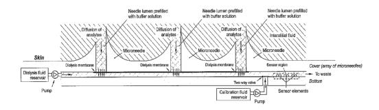
(57) Abstract: A method and apparatus for forming microneedles and other microstructures using hardenable materials and useful for substance monitoring and/or drug delivery.
