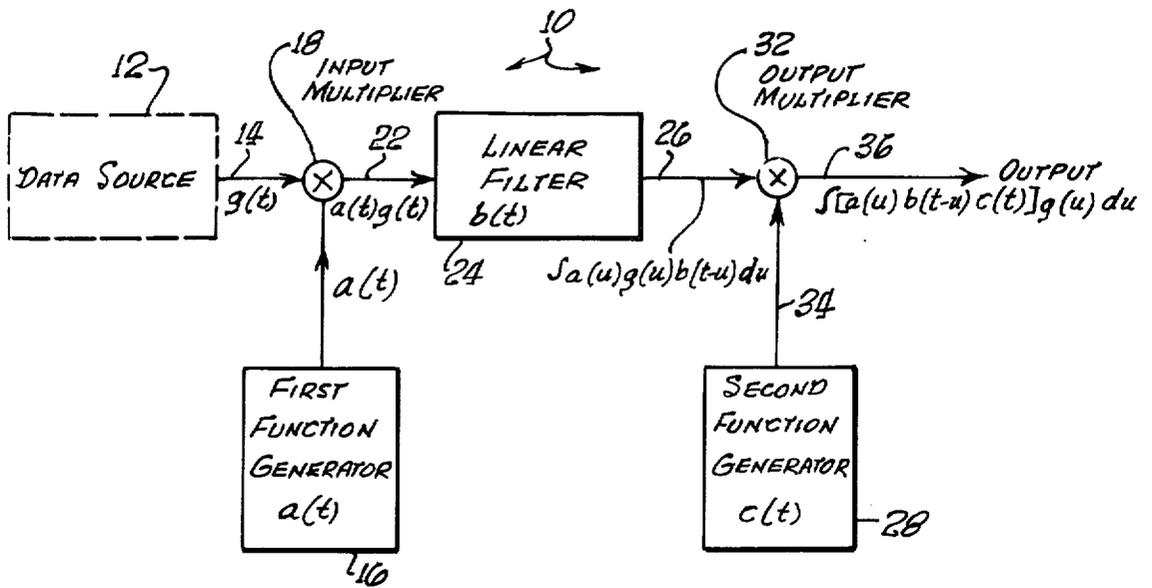
**FIG. 1.** SERIAL-ACCESS APPARATUS FOR THE GENERATION OF A LINEAR TRANSFORM (FILTER FORM)
