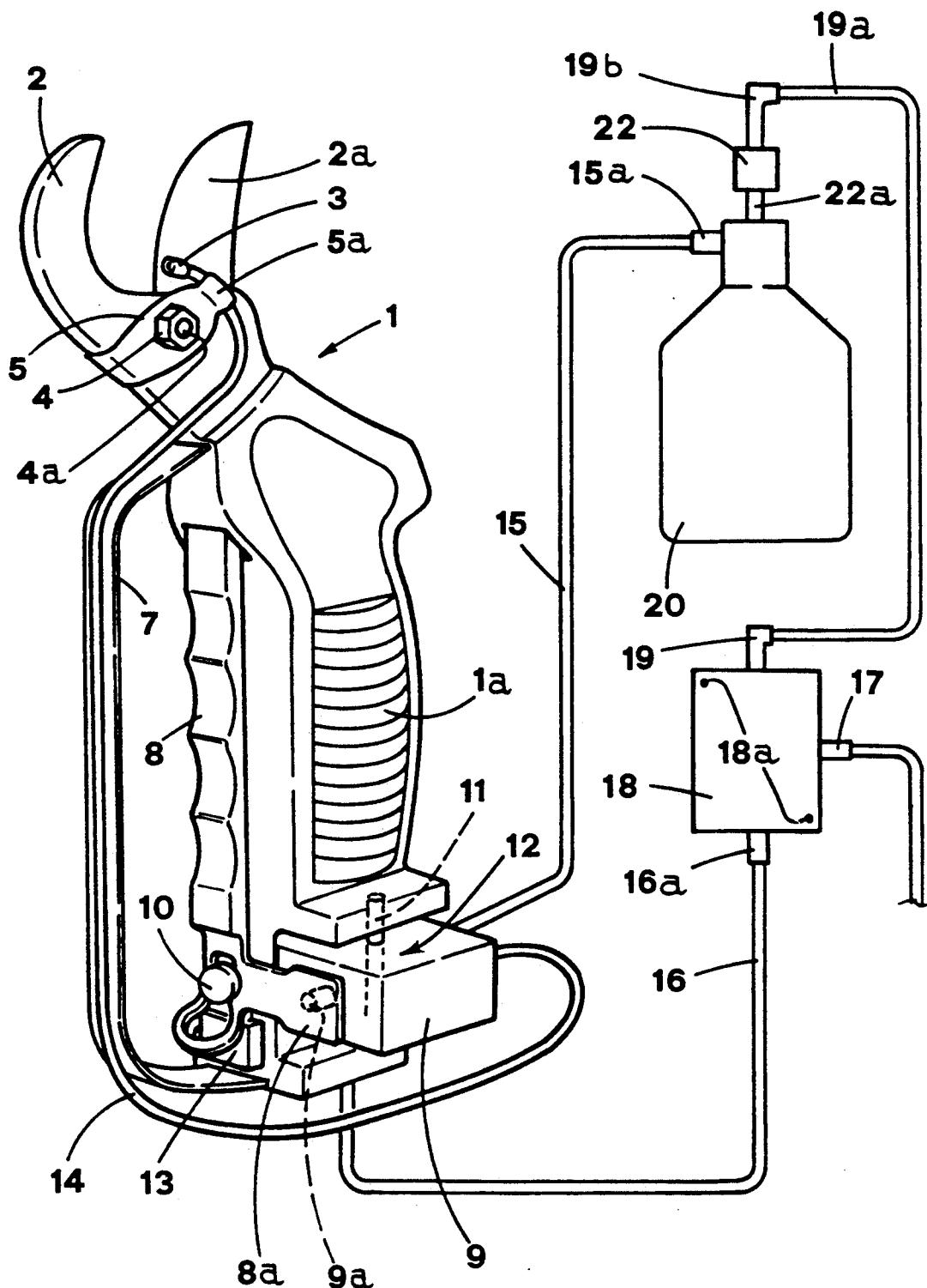
**DEVICE FOR THE DISINFECTION OF PRUNED BRANCHES OR VINE-SHOOTS, APPLIED OR APPLICABLE TO PNEUMATIC SHEARS**
