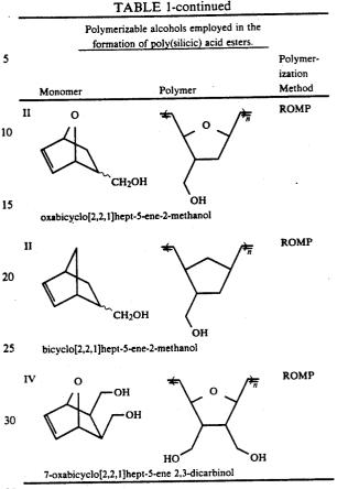
The esterification reaction of poly(silicic) acid with an alcohol, wherein an --OH group of the acid is replaced by an --OR group of the alcohol, results in a 40 poly(silicic) acid ester (PSAE) which has the general formula
