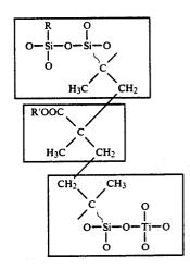
Wei, Y. et al (1990 Chemistry of Material 2, 337-339) reported the synthesis of composite materials by cocondensation of tetraethoxysilane with acrylate polymers containing triethoxysilyl groups. The resulting and silicic groups.
