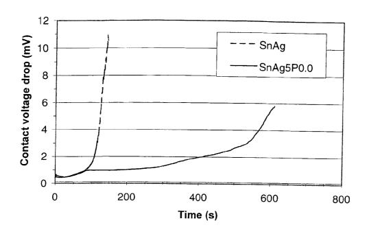
(57) Abstract: The invention relates to a tin alloy coating in a connector for electric contact purposes, such as in contact terminals. The tin alloy coating of the invention is alloyed with at least one reducing agent to achieve an essentially oxide free metal-to-metal contact.
