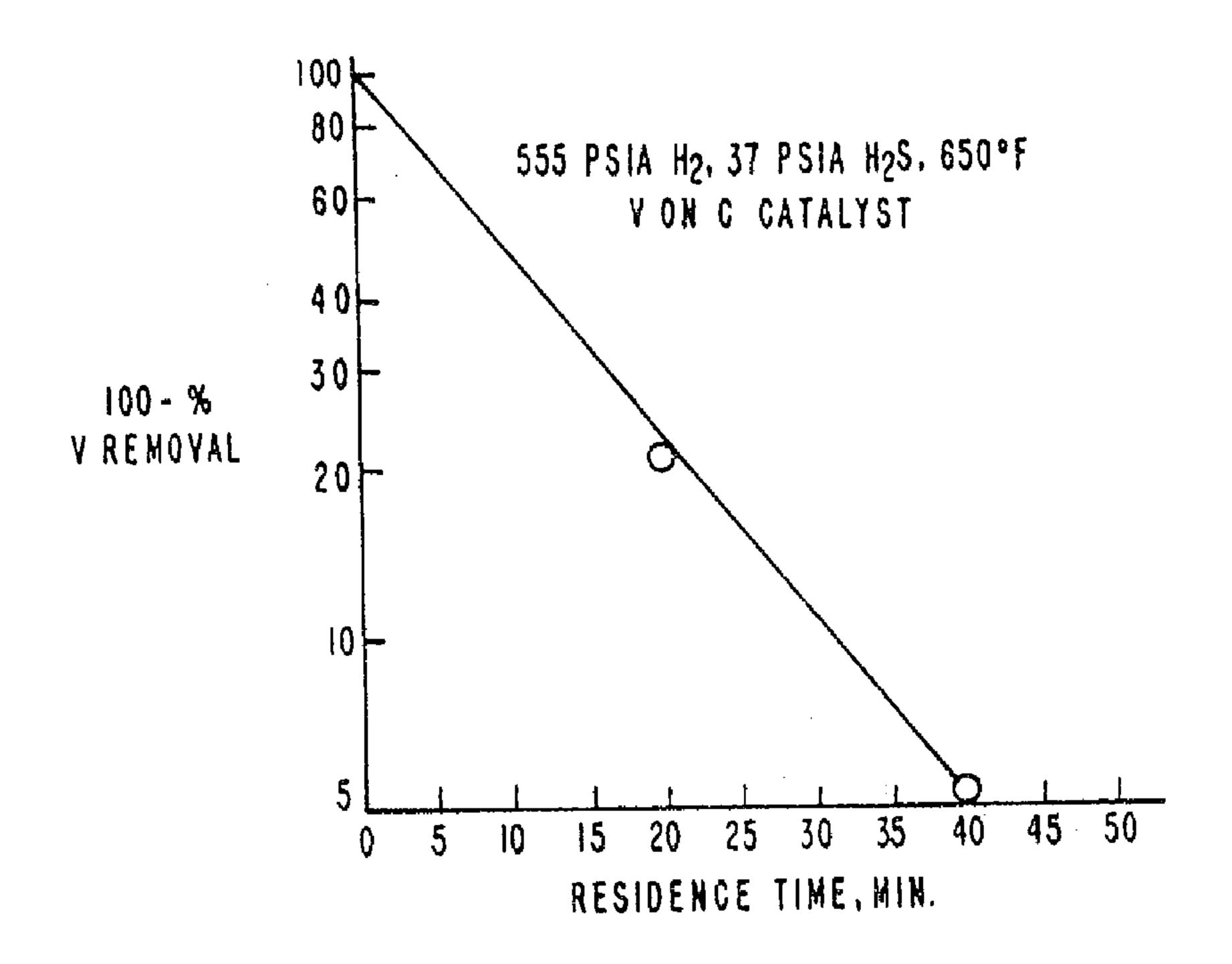
(57) A method of reducing the concentration of metal contaminants, such as vanadium and nickel, in a petroleum distillate or other hydrocarbonaceous liquid is disclosed. The method comprises demetallizing the distillate over an activated-carbon supported vanadium catalyst.
