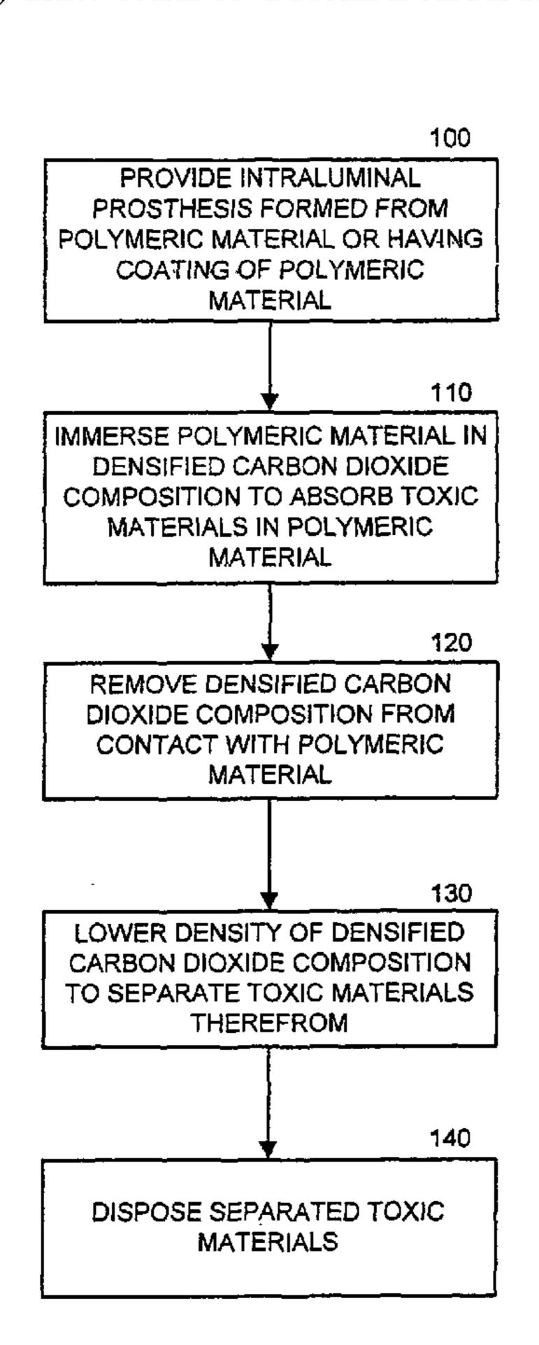
(57) Abstract: Methods of producing biocompatible intraluminal prostheses are provided and include immersing polymeric material of an intraluminal prosthesis in a densified carbon dioxide composition under controlled conditions such that toxic materials are absorbed by the densified carbon dioxide composition.
