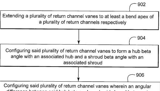
Configuring said plurality of return channel vanes wherein an angular difference between said hub beta angle and said shroud beta angle first decreases, reaching a minimum, then increases, reaching a maximum, then decreases again as you travel along a flow path of said plurality of return channels respectively
