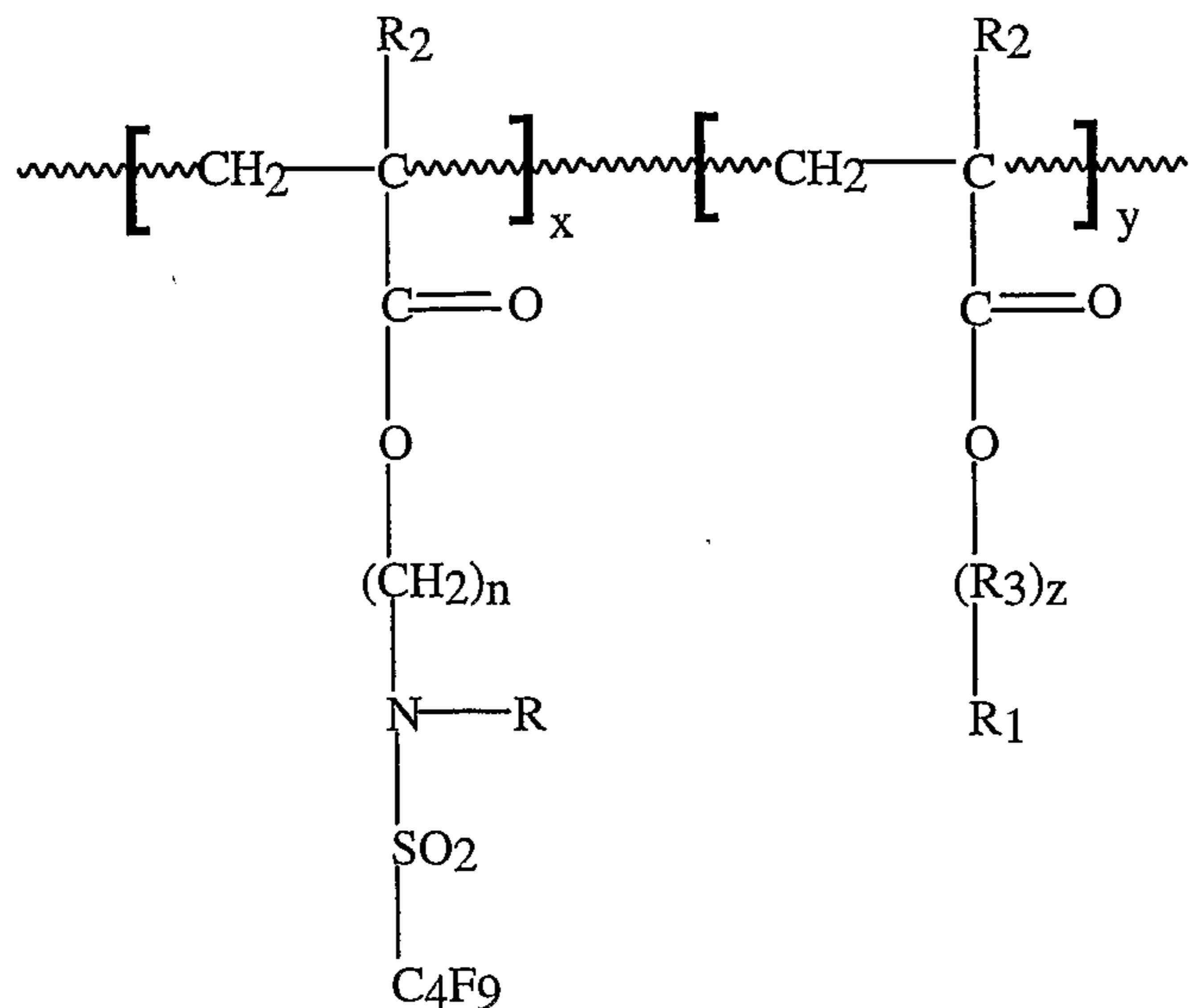
wherein ~~~~~ represents a bond in a polymerizable or polymer chain; R, R<sub>1</sub> and R<sub>2</sub> are each independently hydrogen or alkyl of 1 to 4 carbon atoms; R<sub>3</sub> is at least one or more straight or branched alkyleneoxy groups, linked together and having 2 to 6 carbon atoms, or a straight or branched alkylene group having 12 to 20 carbon atoms; n is an integer from 2 to 10; and x, y and z are integers of at least 1.
