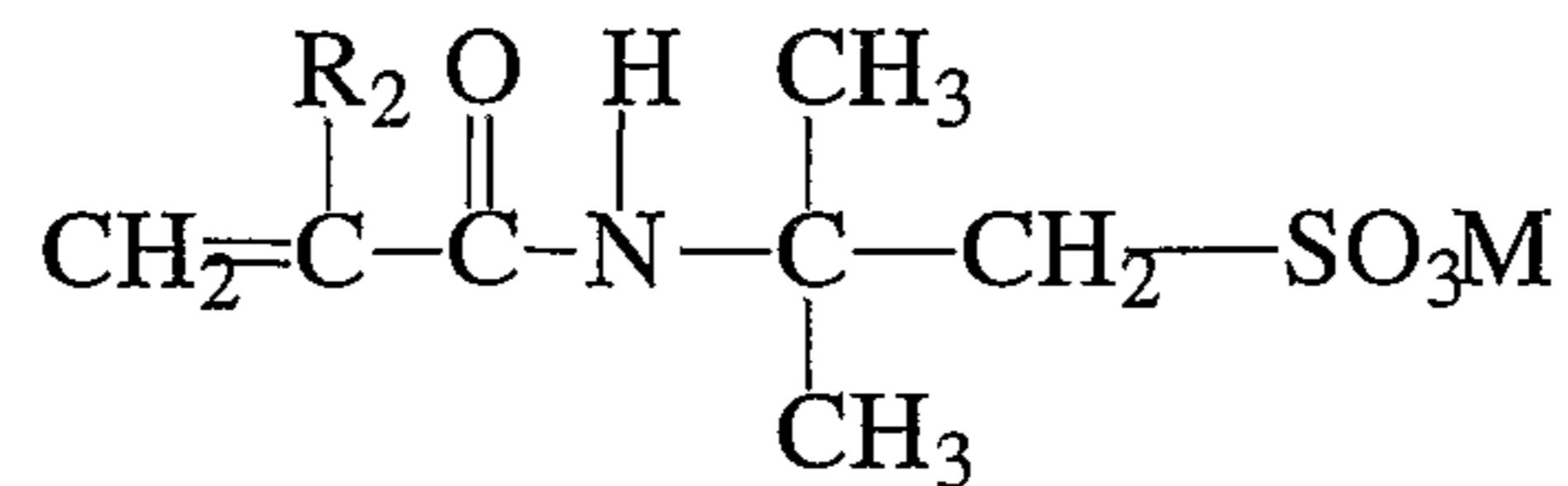
wherein R<sub>2</sub> is hydrogen or methyl and M is hydrogen, potassium, ammonium, lithium, or a protonated tertiary 10 amine.
