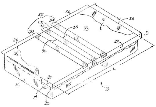
(57) Abstract: A posturized foam topper pad (12) for use in a bedding or seating product (10) has at least one section (28) which includes latex, and at least one section (26) which is free of latex, thereby providing the foam topper pad (12) with different degrees of firmness.
