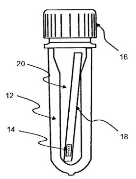
(57) Abstract: A test strip, methods for making and using the test strip, and a kit are described, which allow for the simple and efficient determination of the acetaldehyde content in a polyester polymer. The strip and methods have application, for example, in the manufacture of polyethylene terephthalate preforms and containers, where existing methods for testing for acetaldehyde are cumbersome and time consuming.
