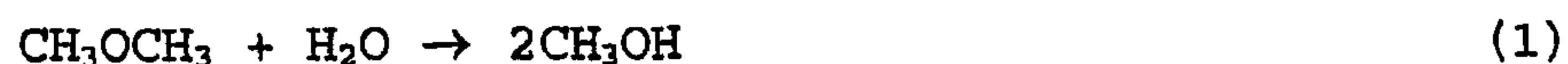
The hydration reaction may take place in either gaseous or liquid phase. Methanol produced during hydration of DME is in a second step decomposed to carbon oxides and hydrogen:
