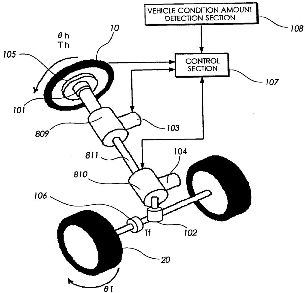
**ELECTRIC POWER STEERING APPARATUS****BACKGROUND OF THE INVENTION**
