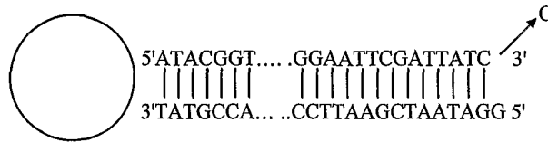
Figure 6C) The single nucleotide overhang at the 5' end is read when the duplex end is captured in the nanopore under an applied voltage.
