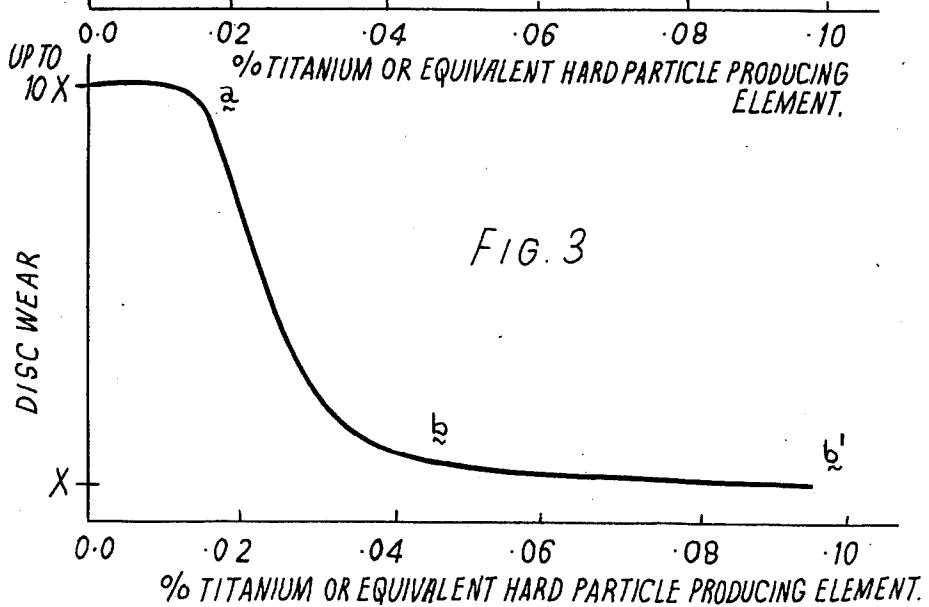
**METHOD OF PRODUCING GREY CAST IRON BRAKE ROTORS WITH UNIFORM FRICTION AND WEAR CHARACTERISTICS**
