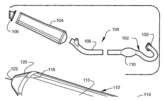
(57) Abstract: A vehicle exhaust assembly (100) for improved evacuation of exhaust gases from an internal combustion engine. The system comprises a modular replacement exhaust system having a novel header pipe (102) and muffler (104). The present invention readily adapts to a range of vehicle applications including automobiles, motorcycles, and all terrain vehicles.
