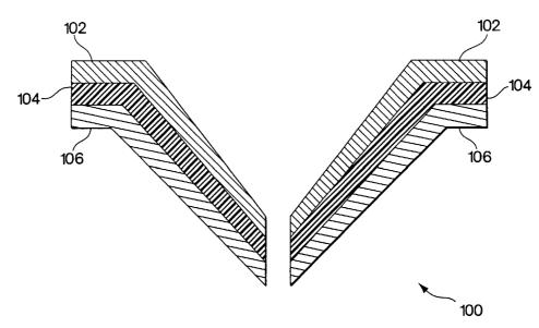
(57) Abstract: The microneedle devices (100) disclosed herein in some embodiments include a substrate (104); one or more microneedles; and, optionally, a reservoir for delivery of drugs or collection of analyte, as well as pump(s), sensor(s), and/or microprocessor(s) to control the interaction of the foregoing.
