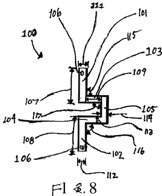
(57) Abstract: A spinal implant (100) comprises a plurality of contiguous segments (101, 102, 103, 104, 105), said plurality of contiguous segments configured to apply a torque to a degenerate spinal segment (18) in any of three orthogonal axes. At least one mounting connection (106) is configured to connect said spinal implant to a mounting mechanism (202), said mounting mechanism being configured to attach said spinal implant to said degenerate spinal segment.
