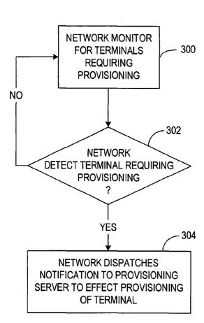
(57) Abstract: The network monitors (300) for terminals that have not been provisioned for connection to a network or service, automatically detects and recognizes (302) a terminal requiring provisioning, and dispatches (304) a notification to a provisioning server to effect such provisioning of the terminal when an unprovisioned terminal has been detected.
