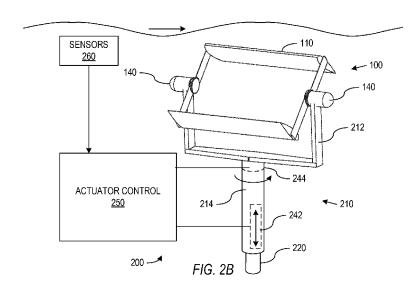
(57) **Abstract**: A system for mounting a set of wave energy converters in the ocean includes a pole (220) attached to a floor of an ocean and a slider (210) mounted on the pole (220) in a manner that permits the slider (210) to move vertically along the pole (220) and rotate about the pole (220). The wave energy converters (100) can then be mounted on the slider (210) to allow adjustment of the depth and orientation of the wave energy converters (100).
