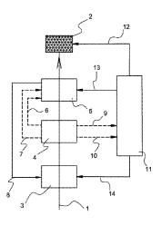
particular the yarn clearer (5), and with regard to the yarn length and/or the yarn speed are provided to the machine controller (11).
